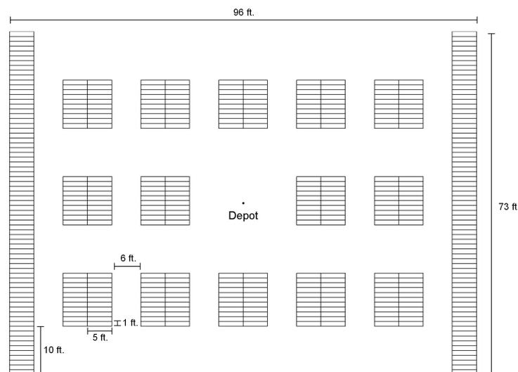
(b) A warehouse with a central depot, 6 PAs and 4 CAs. There are 454 storage locations in this 651-square-meter facility, identified as Layout 15 in Table 3.
