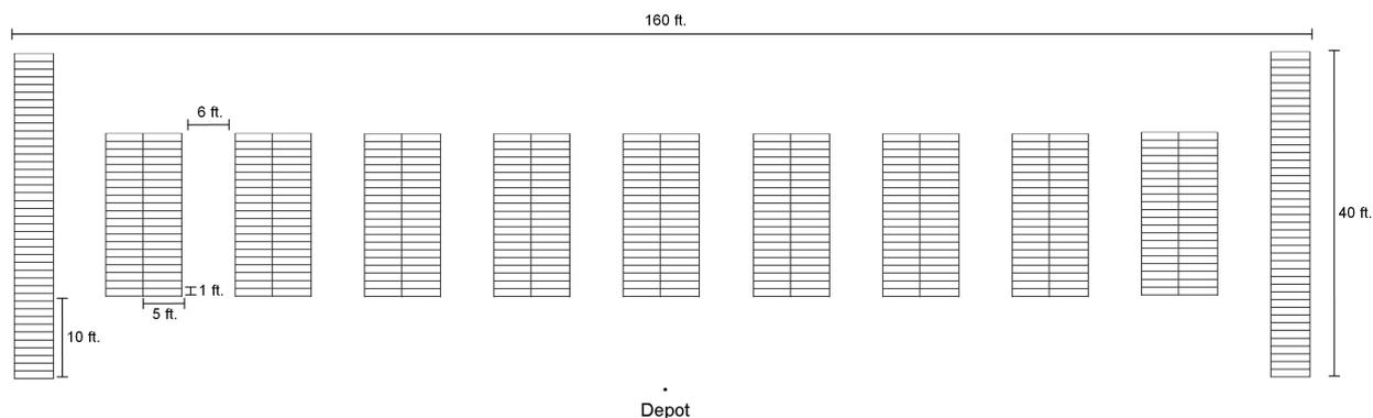
(a) A warehouse with a traditional depot, 10 PAs, and 2 CAs. There are 440 storage locations in this 595-square-meter facility, identified as Layout 7 in Table 3.
