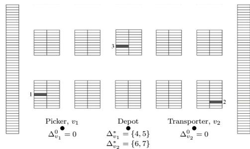
(a) An example warehouse layout showing three pick locations ( $I = \{1, 2, 3\}$ ), a picker and a transporter. Both the picker ( $v_1$ ) and transporter ( $v_2$ ) start at node 0, although the vehicles are in different physical locations.
